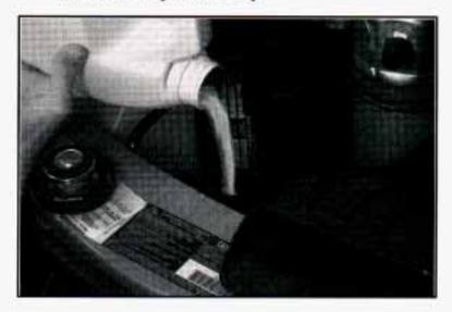
3. Fill the radiator with the proper mix, up to the base of the filler neck.
